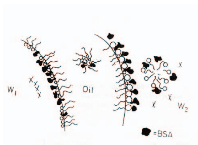
Figure 14 Schematic illustration of possible organization and stabilization mechanism of BSA and monomeric emulsifiers (Span 80) at the two interfaces of double emulsion.
